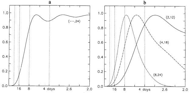
Fig. 1. Response of highpass (a) and bandpass (b) filters used in this study.
