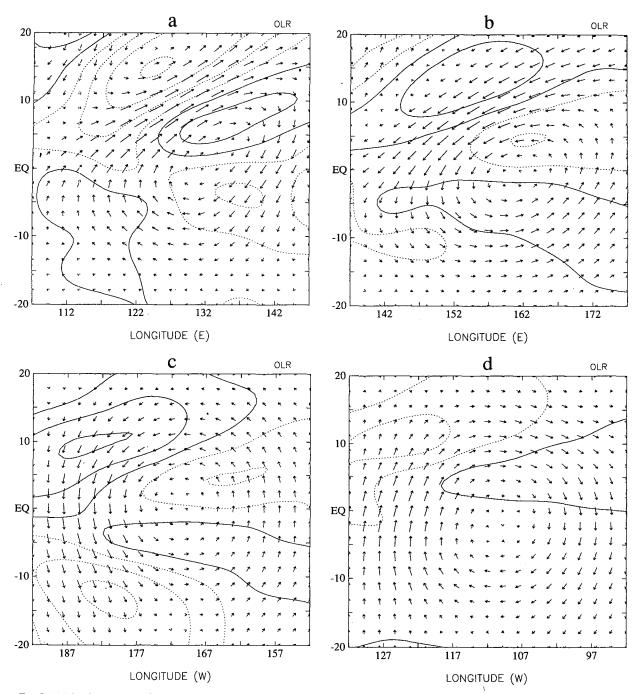
Fig. 9. Multivariate horizontal EOFs from 700-mb ECMWF and OLR data, based on the correlation matrix of horizontal wind components (vectors) and OLR (contours). (a) Far western Pacific; (b) west-central Pacific; (c) east-central Pacific; and (d) far eastern Pacific. Contour interval for OLR is 0.10, starting at ±0.05. The longest vector corresponds to a nondimensional EOF value near 0.6.
