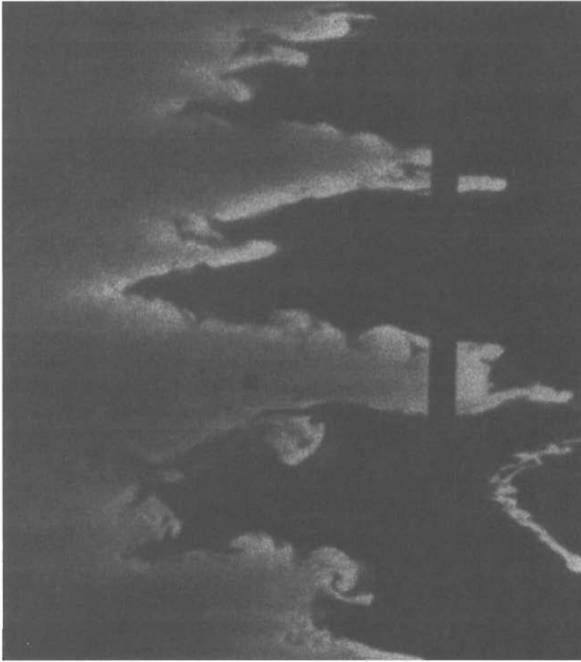
Figure 5 Turbulence collapse and intrusion formation; \omega/N \approx 72 , Nl = 25.4 (Browand et al 1987).
