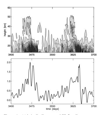
**Figure 4.** (a) latitudinally averaged EP flux divergence, as a function of height and time for a representative subinterval of the model integration; (b) latitudinally averaged upward EP flux through 200 hPa as a function of time for the same subinterval. The contour interval in (a) is  $10^{14}$  kg m s<sup>-2</sup>, with negative values (convergence) shaded and darker tones corresponding to larger negative values. Units in (b) are  $10^{19}$  kg m<sup>2</sup> s<sup>-2</sup>.
